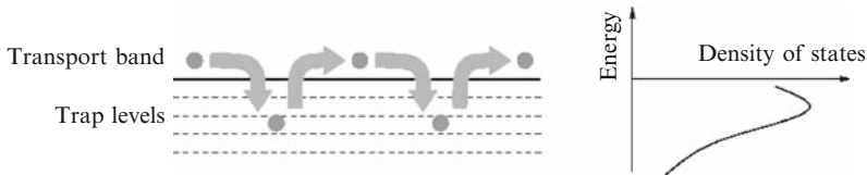
Fig. 4 Principle of the multiple trapping and thermal release limited charge transport
